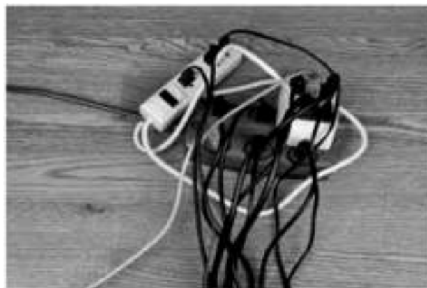
Fig. 11.2: Overloaded power strip.
