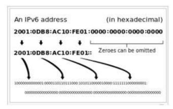
Figure 4: Decomposition of an IPv6 address from hexadecimal representation to its binary value<sup>4</sup>
