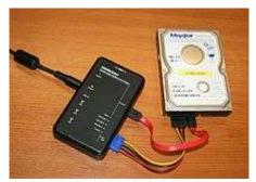
Figure 56: A portable Tableau write blocker attached to a Hard Drive<sup>79</sup>
