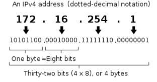
Figure 3: IPv4 address
