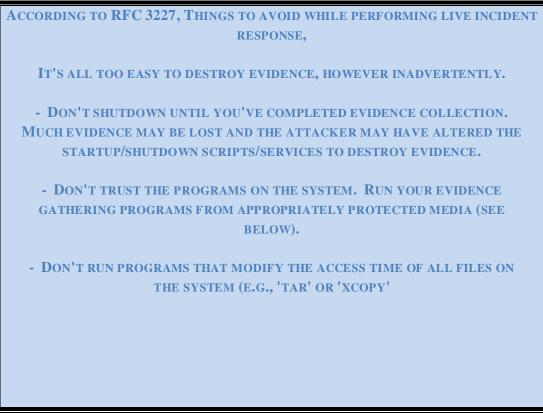
Figure 36: RFC 3227 guidelines for live incident response
