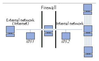
Figure 5: An intrusion detection system<sup>14</sup>
