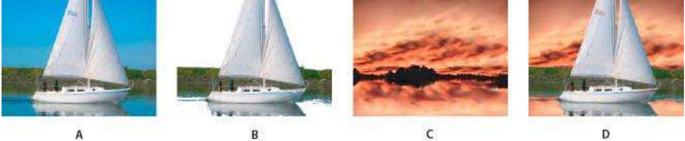
A. Original image B. Blue color keyed out C. Image on second track D. Final composite image
