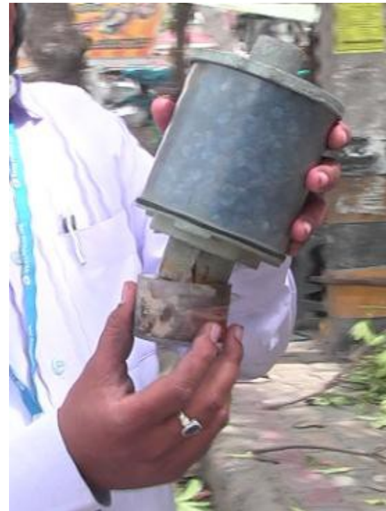
Fixing the oil cup to breather
