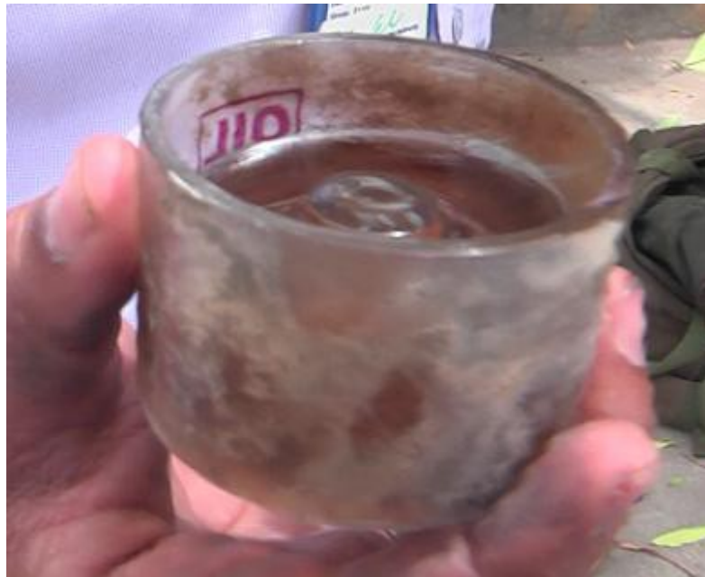
Breather oil cup is filled with fresh oil
