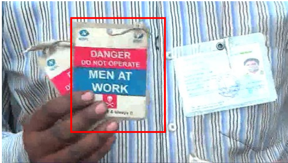
‘Do Not Operate Tag’ – Tag to be used when electricity is shut down
