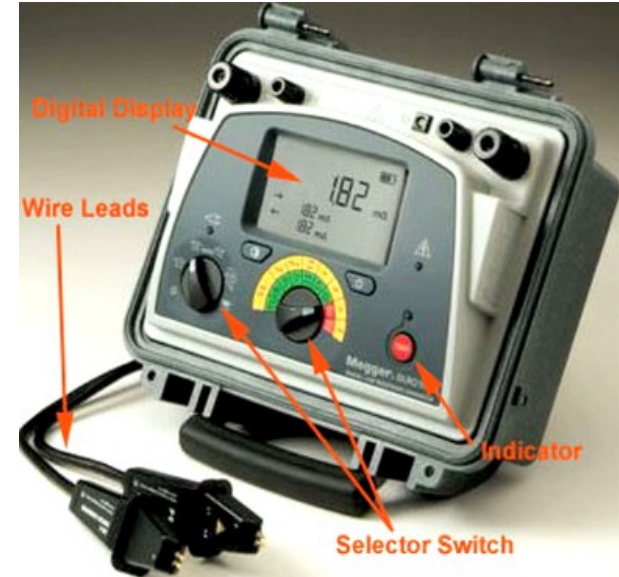
Instrument that pin points the cable fault
