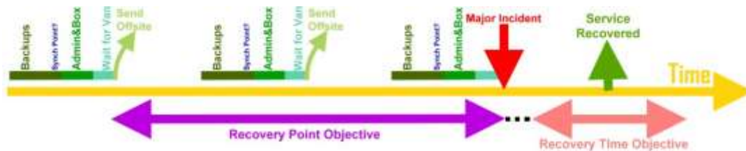
Figure 13: A DR plan illustrating the chronology of the RPO and the RTO with respect to the MI
