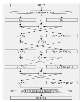
Figure 65: DES enciphering algorithm
