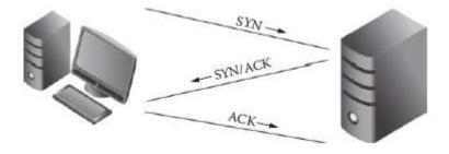
Figure 93: TCP three way handshake
