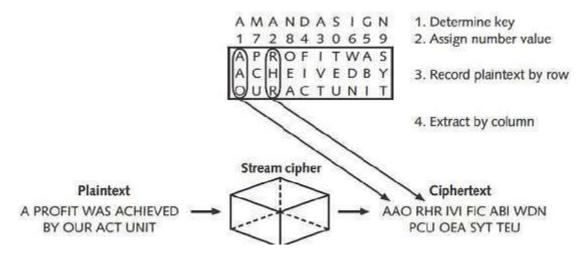
Figure 24: Transposition Cipher
