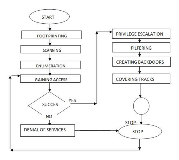
Figure 45: Sequence of Pen Testing/ Hacking
