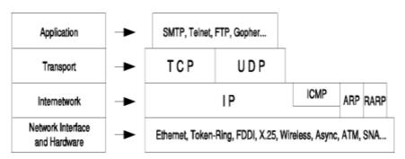
Figure 4: TCPIP protocol suite and compatible protocol at each layer
