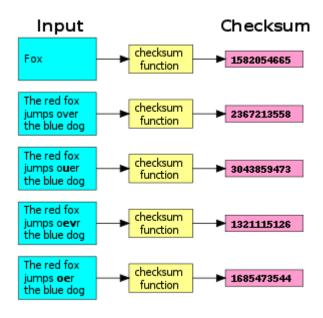
Figure 67: Effect of a typical checksum function (the Unix cksum utility)
