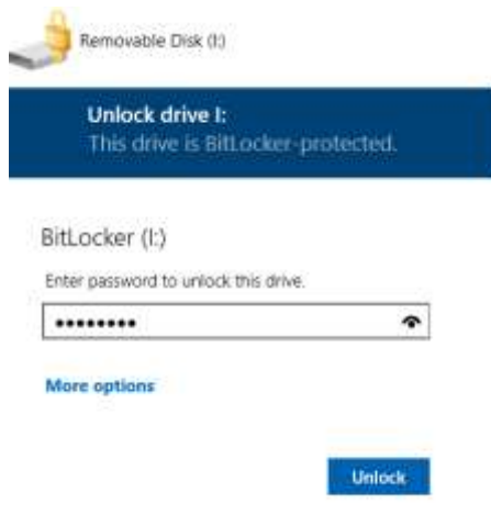
Figure 62: Unlocking the encrypted drive using password
