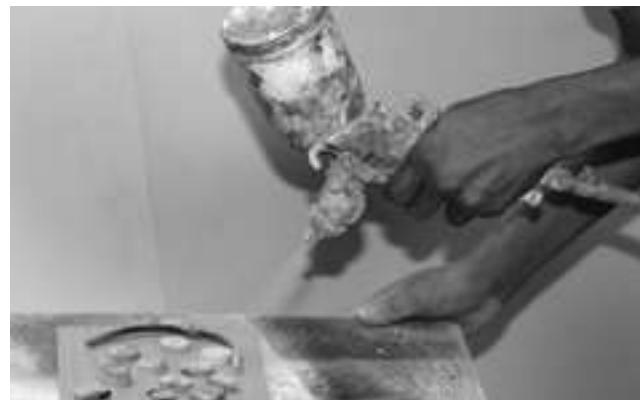
Step 9: Finish it with mellamine before the assembly.
