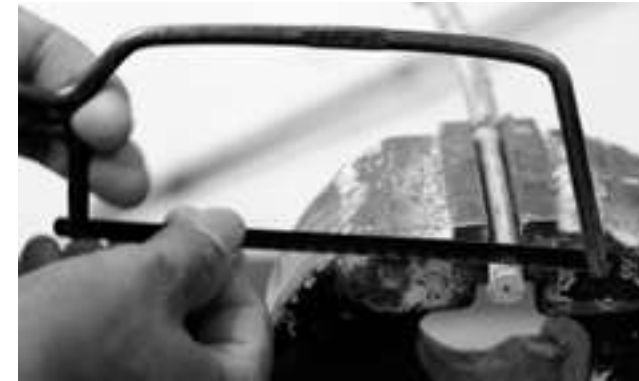
Step 1: Cut the bamboo branches into small pieces using hacksaw
