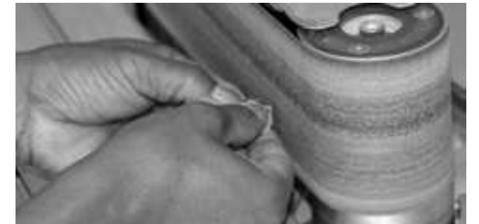
Step 5: Finish on the sanding machine.
