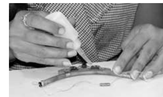
Step 16: Use an adhesive to stick the components.
