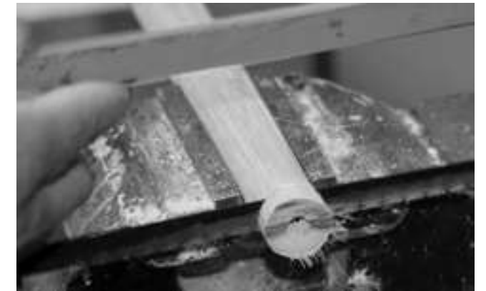
Step 4: Cut the solid bamboo to make beads.
