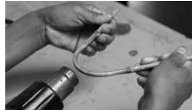
Step 2: Bend the branches using hot air gun
