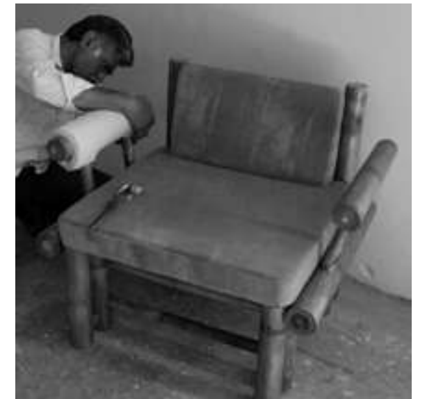
Step 10: Fixing the upholstery to the sofa frame.
