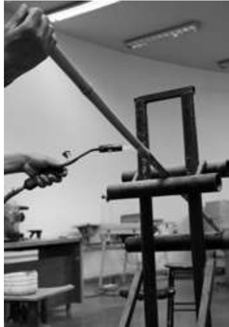
Step 1: Straightening solid bamboo by heating and pushing on jig
