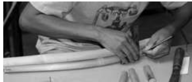
Step 4: Mark points on bamboo for drilling.
