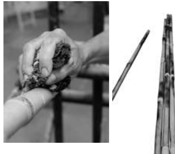
Step 3: Cooling the surface of bamboo with water
