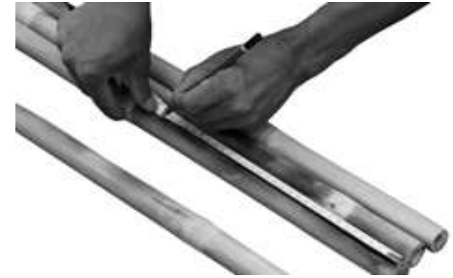
Step 8: Make a 30 cms mark on the bamboo
