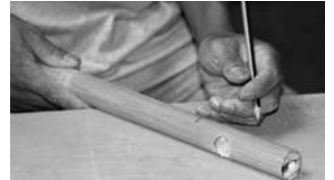
Step 20: Make a leg member and mark it for drilling a hole through it
