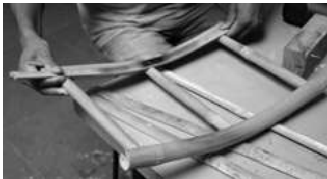
Step 13: Match the curve with frame.
