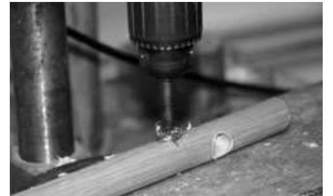
Step 21: On the leg unit, drill the hole for fixing the tie member.
