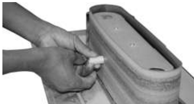
Step 13: Sand the edges to smoothen it
