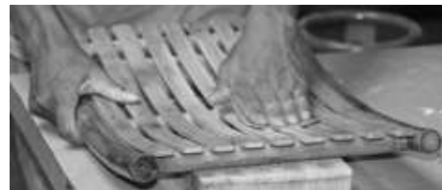
Step 19: After fixing it use sand paper to finish the surface
