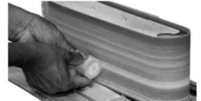
Step 4: Using a sander, smoothen the surfaces
