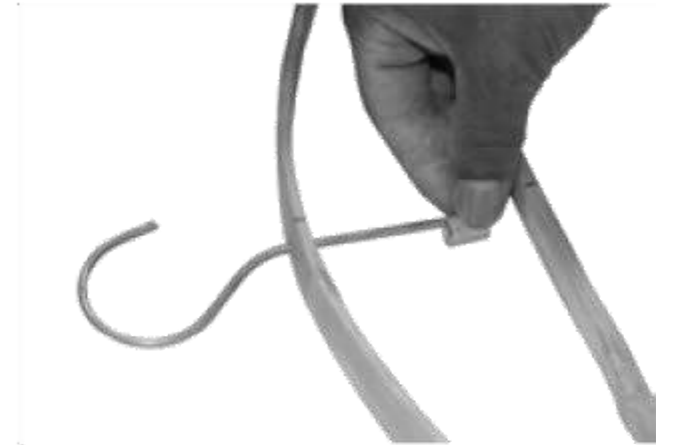
Step 8: Drill a hole through top sliver
