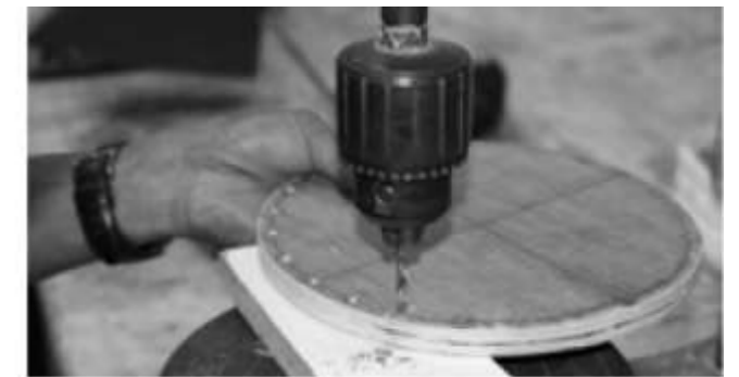
Step 5: With a 3-4mm drill bit, drill holes on marks
