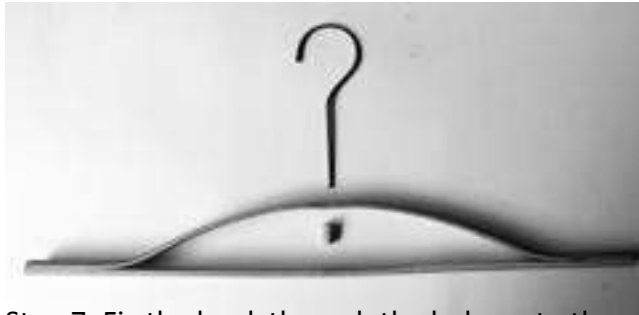
Step 7: Fix the hook through the hole on to the topper bead.
