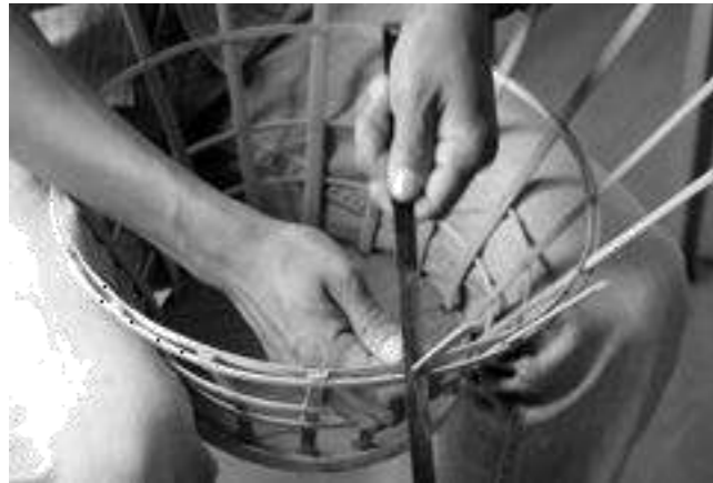
Step 18: Cut excess length of the slivers
