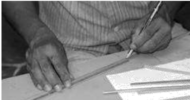
Step 7: Mark 30 cm lengths on the slivers.
