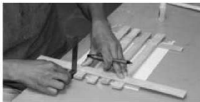
Step 6: Mark and align it with the paper edge.
