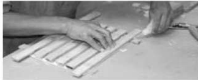
Step 4: Stick the splits using an adhesive
