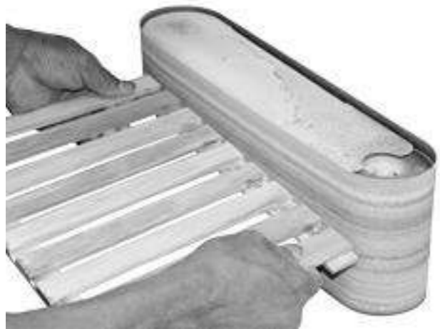
Step 12: Use a grinder to smoothen the edges.
