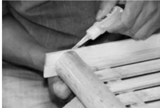
Step 14: Fix another sliver perpendicular to the tray
