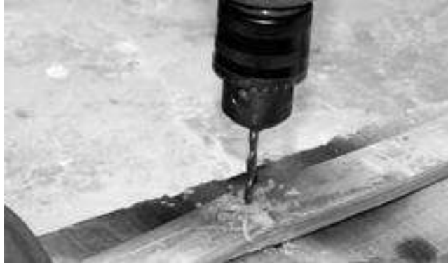
Step 6: Drill the hole in the center of the top sliver
