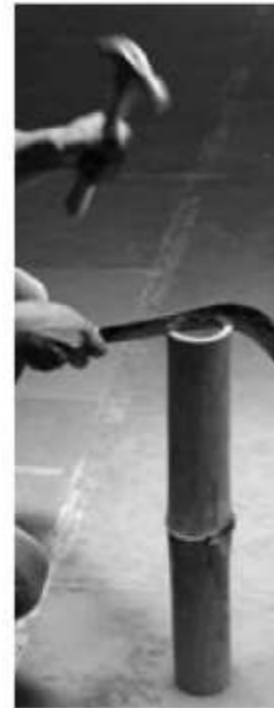
Step 1: Split the bamboo to thick sliver.
