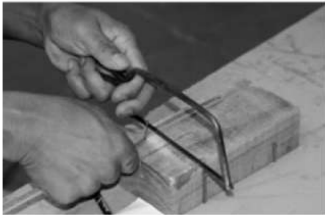
Step 8: Cut the slivers on the mark to get equal length inside.
