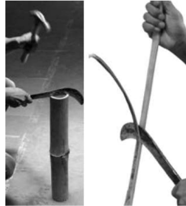
Step 1: Splitting the bamboo to thick slivers.
