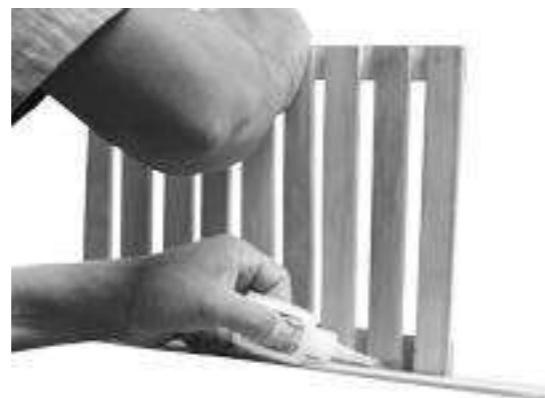
Step 15: Mark equal distances on the extended ends
