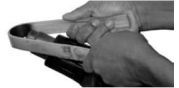
Step 3: Bend two slivers into U shaped curves and fix them using glue to flat ends of the first sliver
