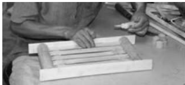
Step 15: Attach with adhesive on both sides
