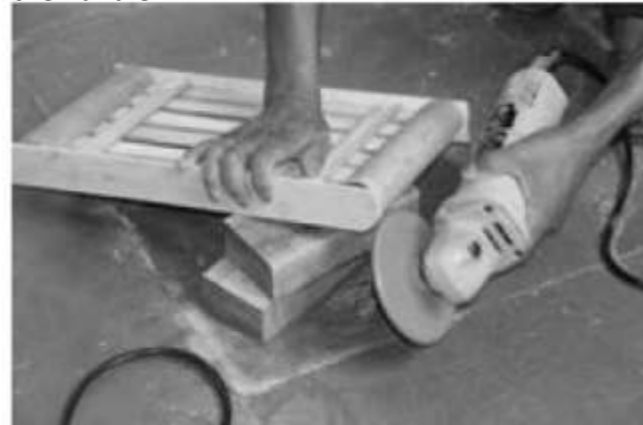
Step 17: Grind the split along the handle.
