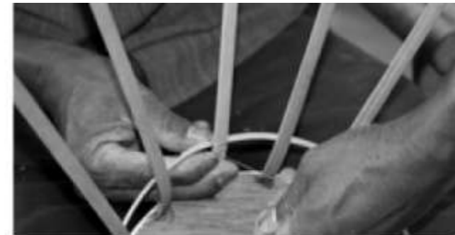
Step 13: Tie the ring using thin copper wire.
