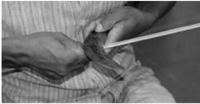
Step 6: Make thick slivers of reed bamboo and bend the bamboo slivers at one end.
