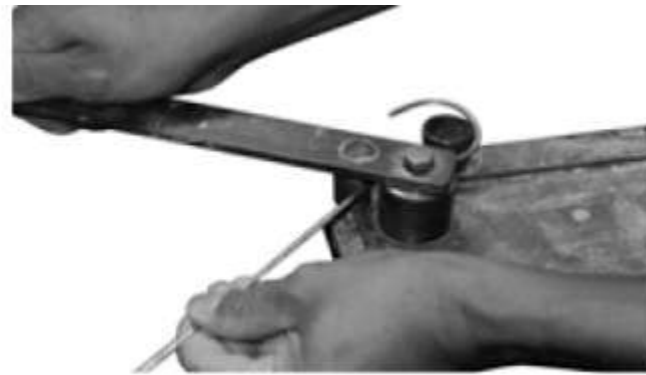
Step 7: Bend the S. S rod into shape of a hook
