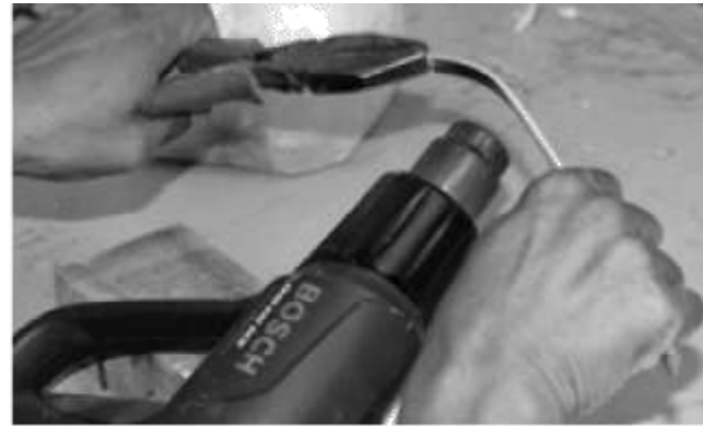
Step 6: Make thick slivers of reed bamboo and bend the bamboo slivers at one end.
