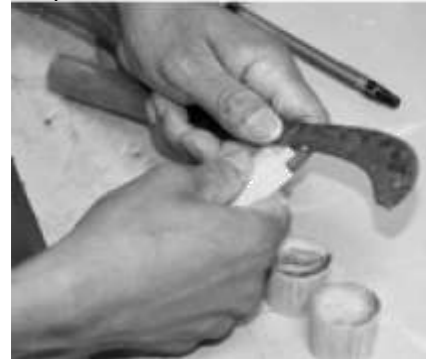
Step 7: Make a notch on hanger ends, the same diameter as the hole in the solid bamboo
