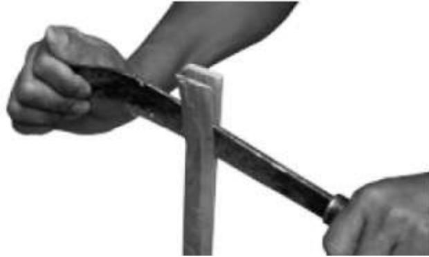
Step 1: Split the bamboo to thick and wide splits.
