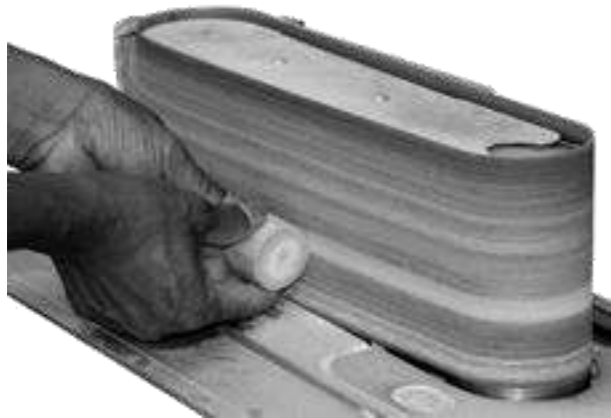
Step 5: Sand the rough edges of the bamboo piece
