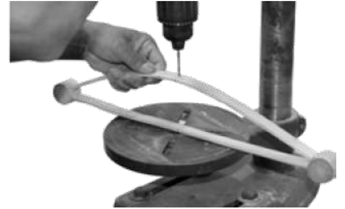
Step 8: Drill a hole through top sliver
