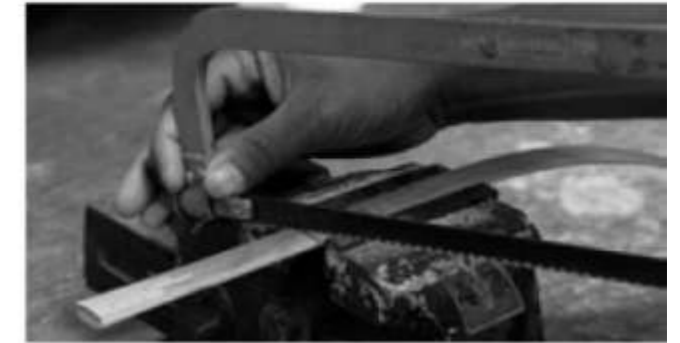
Step 3: Cutting the excess length.
