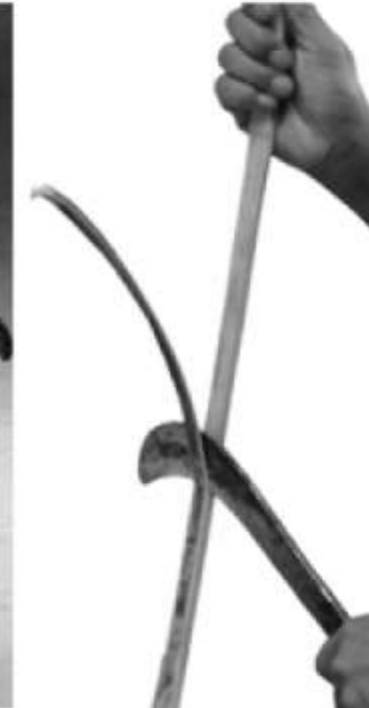
Step 1: Splitting the bamboo to thick slivers.
