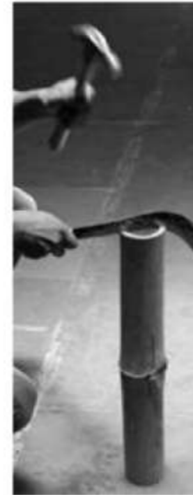
Step 1: Splitting the bamboo to thick slivers.
