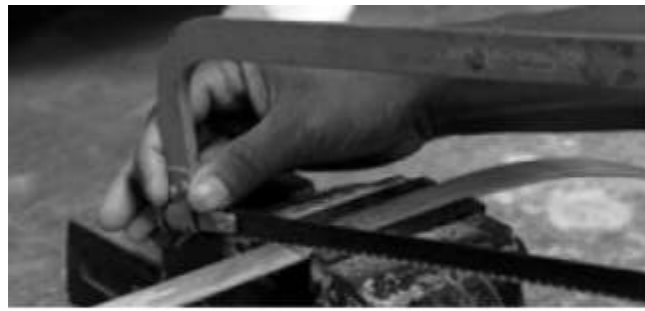
Step 4: Cut the excess length using a hack saw.
