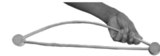
Step 11: Fix a flat, sanded sliver to the second holes of the bamboo
