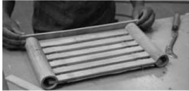
Step 13: Insert the sliver into the notch
