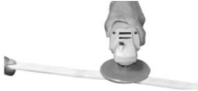
Step 3: Use grinder to make the splits straight and flat.
