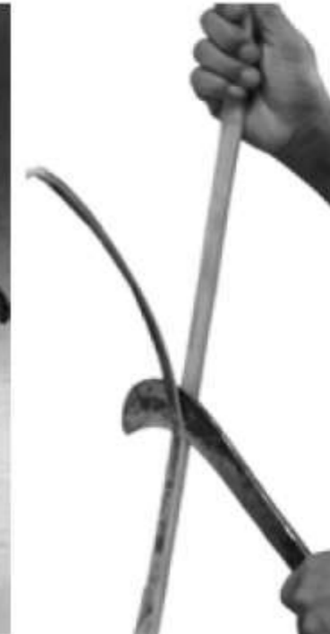
Step 1: Split the bamboo to thick sliver.
