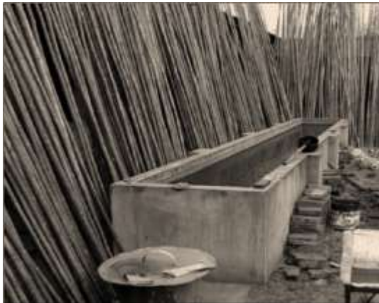
Figure 10: A preservation pool for bamboo culms
