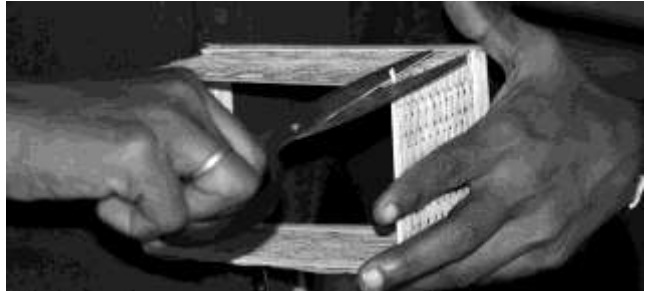
Step 3: Make the mat into a rectangular box shape and cut of the edges
