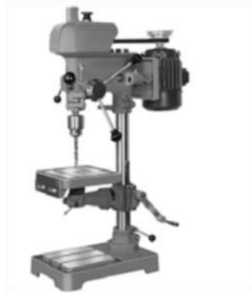
Pillar Drill Used for drilling on the surface of wood, bamboo, metal etc.
