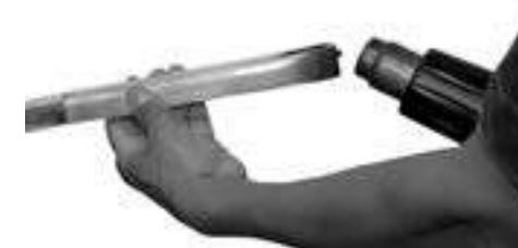
If required (wet or green bamboo) also heat behind the curve on the skin.
