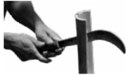
Further splitting of half bamboo to the required width.
