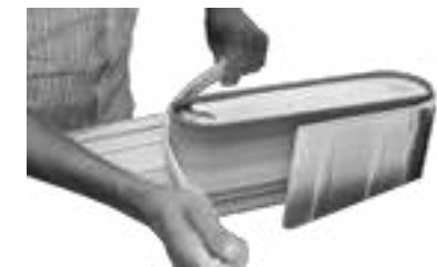
Hold the material tightly while sanding on the sanding machine.
