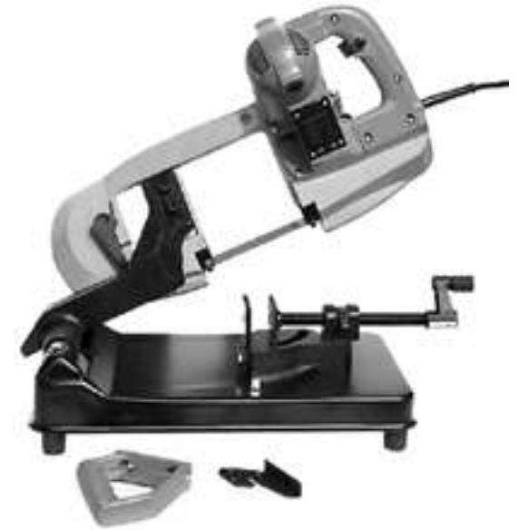
Bench top horizontal band saw Used for cross cutting the bamboo in any angle required.
