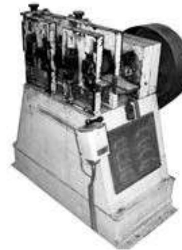
Slivering machine This machine makes thick sliver suitable for making furniture and lifestyle products.
