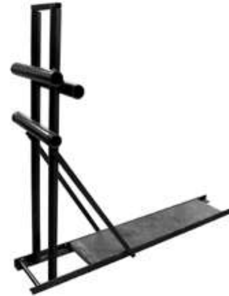
Bending Stand Used as a supporting jig while bending the solid bamboo.
