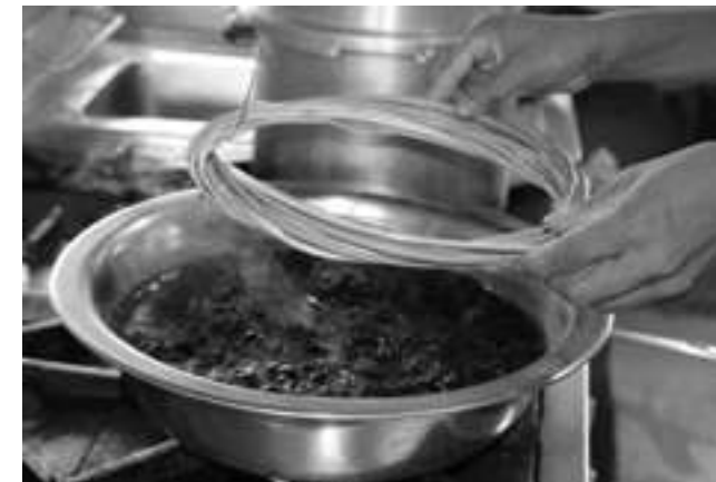
Place the bamboo sliver in the prepared mix.
