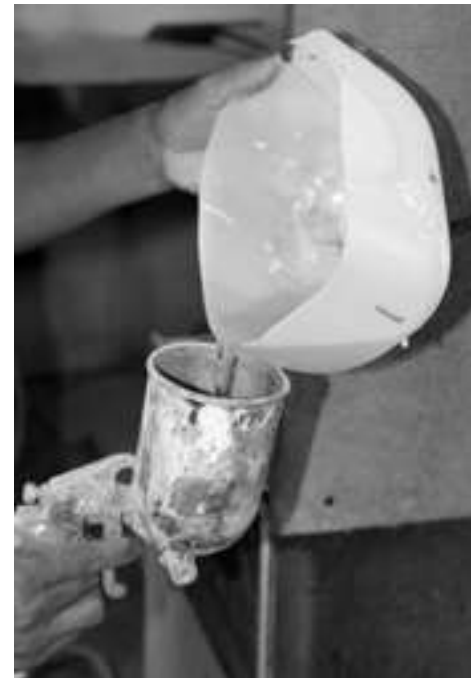
Pour the mixture in the container of airbrush.
