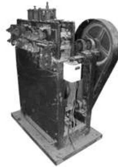
Node removing machine After splitting in radial splitter this machine is used to remove the nodes.
