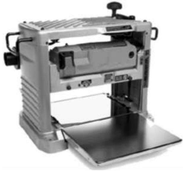
Surface planer Used for levelling the surface of wood or bamboo splits.
