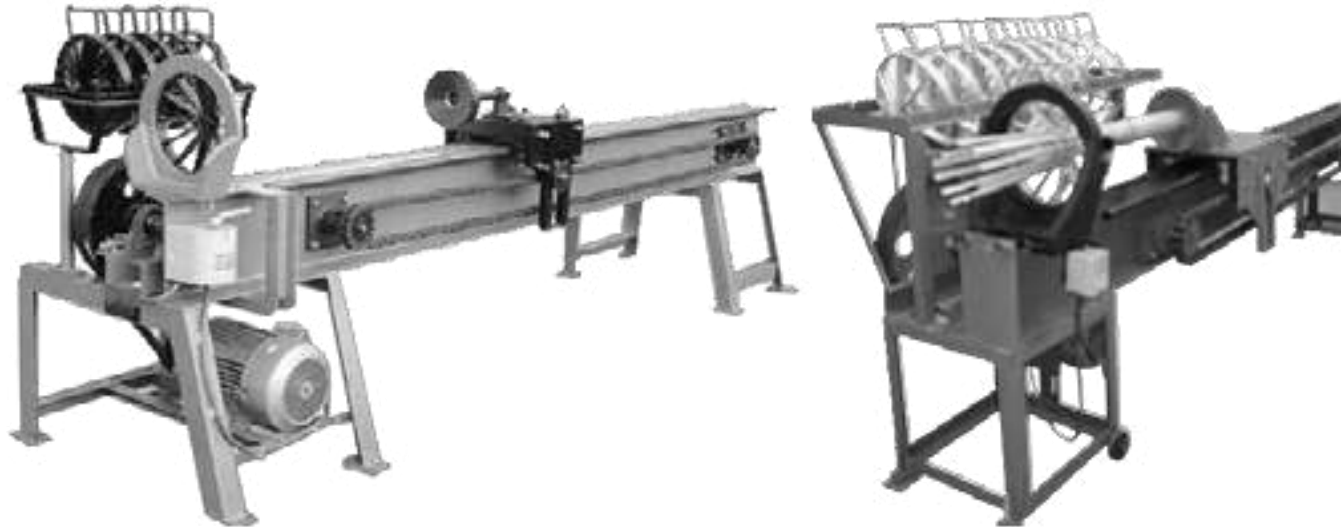
Bamboo radial splitter This machine is used to split the bamboo radially to various numbers as required.
