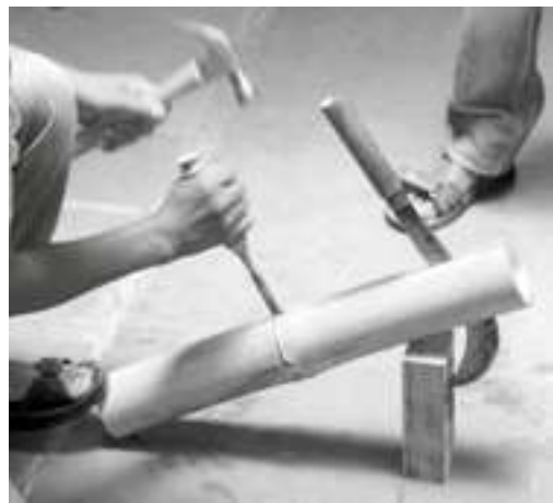
Knife and chisel used with hammer for splitting the bamboo into half
