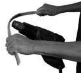
Bending the bamboo split using hot air gun. Start bending by heating the surface.
