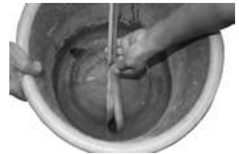
After bending apply water or dip it in the water for cooling the bamboo which helps to retain the shape.
