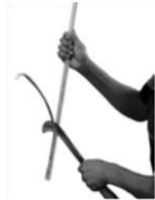
Reducing the thickness of the bamboo by using the knife.
