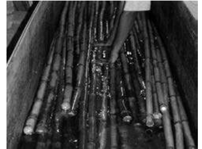
Bamboo poles are placed in the open tank.
