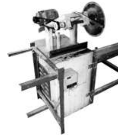
Cross cut saw This machine is used for cutting the length of bamboo.
