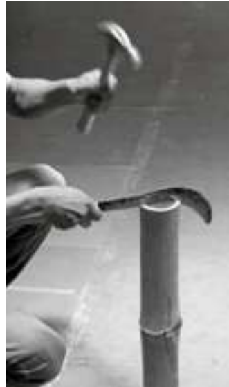
Using a knife and a hammer/mallet to split the bamboo into half.
