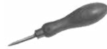
Marking chisel Sharp pointed chisel used for marking the material.
