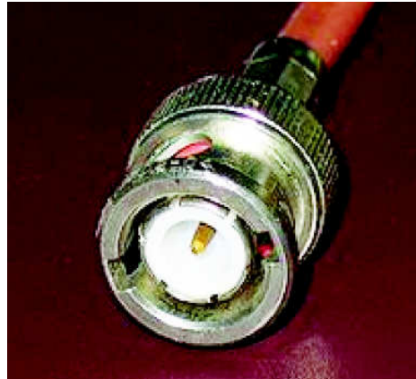
Figure 20.6 (B): BNC (male) type connector
