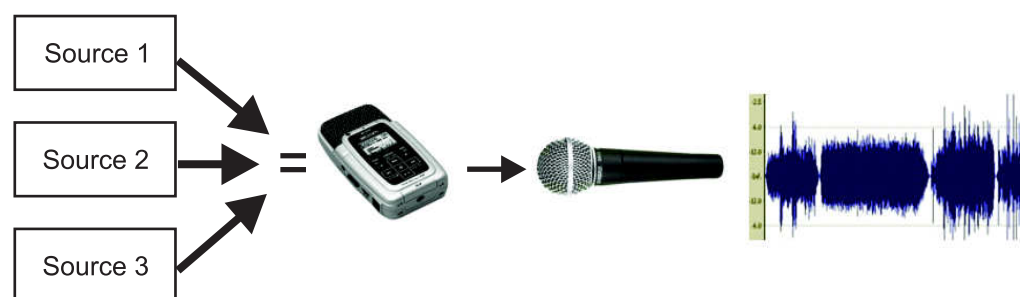
Figure 16.2: Multiple sources recorded on a single microphone, resulting in a mono track. The squiggles are the graphic representation of the audio also known as the waveform display of the audio
