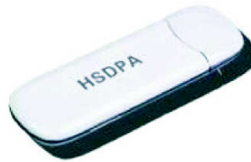
Figure 15.2: A typical GSM dongle unit. HSDPA stands for High Speed Data Packet Access, a type of high speed mobile connectivity protocol. (The screenshot was captured by the author)
