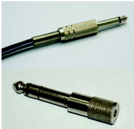
Figure 13.8: 1/4" phono jacks. The one on the left is mono, the one on the right is stereo (Source: Jnan Taranga, KKHSOU, Guwahati)
