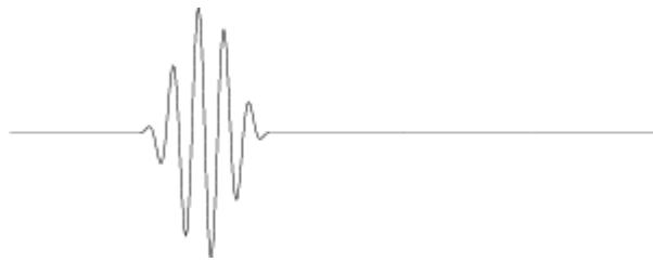
Figure 2.5: A snapshot of a transverse wave on a string. Think of the wave as moving from left to right – but remember that the string is really only moving up and down.
