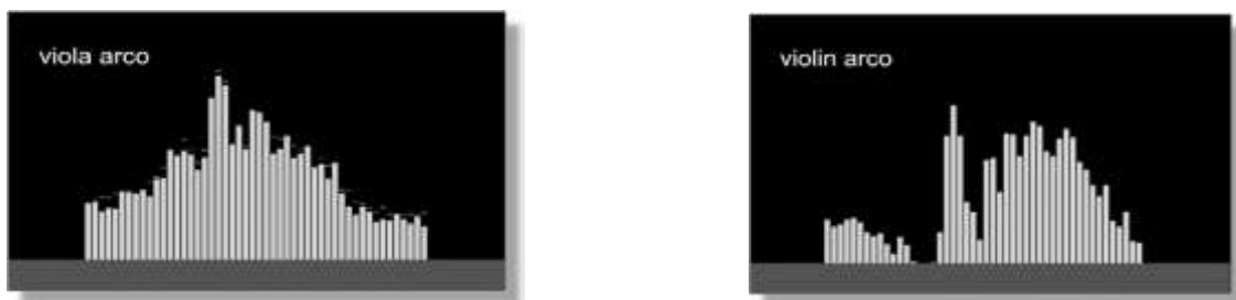
Figure 1.17: Harmonic structure of concert A-440: (a) played on a viola; (b) played on a violin.
