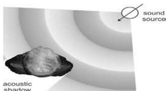
Figure 2.8 The head casts an acoustic shadow that helps with localization at middle to upper frequencies.
